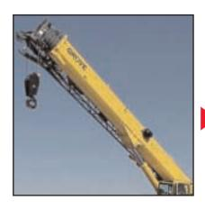
▶ 110 ft. (33.5 m) Four-section full power MEGAFORM™ boom with "quick reeve" boom nose
