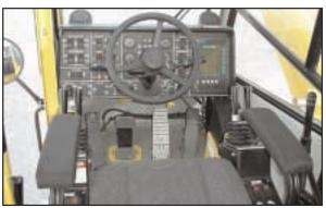
Hot water heater cab with defroster, sliding skylight with sunscreen, armrest-mounted single
